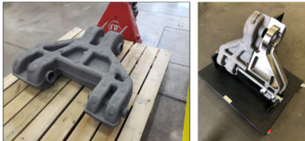
Figure 6 Example of cast canister for the manufacture of civil aerospace primary structure. Casted canister after HIP (left), half machined part (right).
